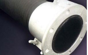
Jachris offers a re-designed split flange coupling – re-useable aluminium couplings suitable for use on hardwall materials handling hoses. Our split flange couplings are ideal for connecting hose to hose, hose to steel pipe or joining a rubber hose to a HDPE pipe.
